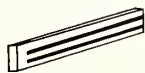
STOCK LESS THAN \frac{6}{4} " THICK SHALL BE SAWED AS SHOWN SO AS TO PRODUCE THREE PRONGS OF EQUAL THICKNESS FOR CASEHARDENING TEST. THE CENTER PRONG SHALL BE BROKEN OUT.
